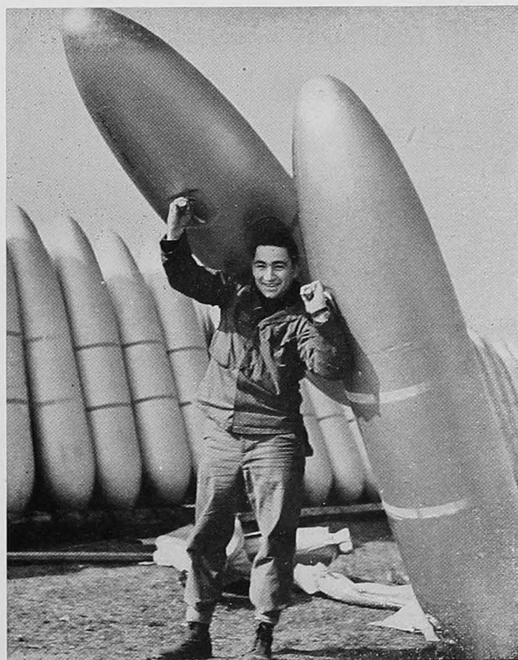
GOERING'S SURPRISE —Luftwaffe Chief Hermann Goering said he sensed doom when U.S. fighters began to soar for hours at a time over Fortress Germany. Pfc. Anthony Rago shows you the reason—those extra-light, extra-range tanks that spelled Wretham to Berlin and return.
