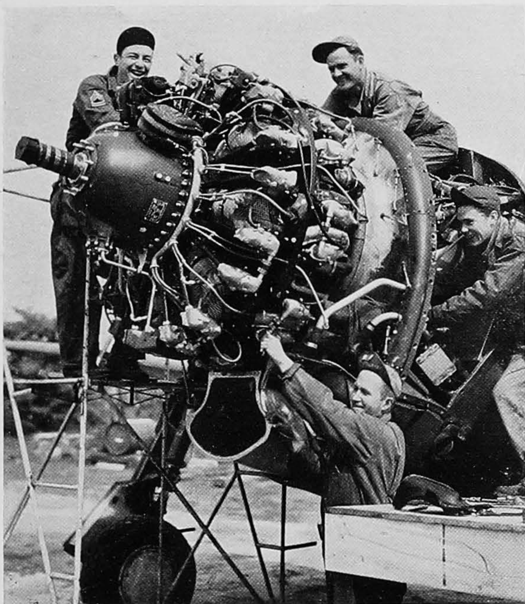
WHEN A P-47 radial engine shed its cowl, it was easily gotten at.
