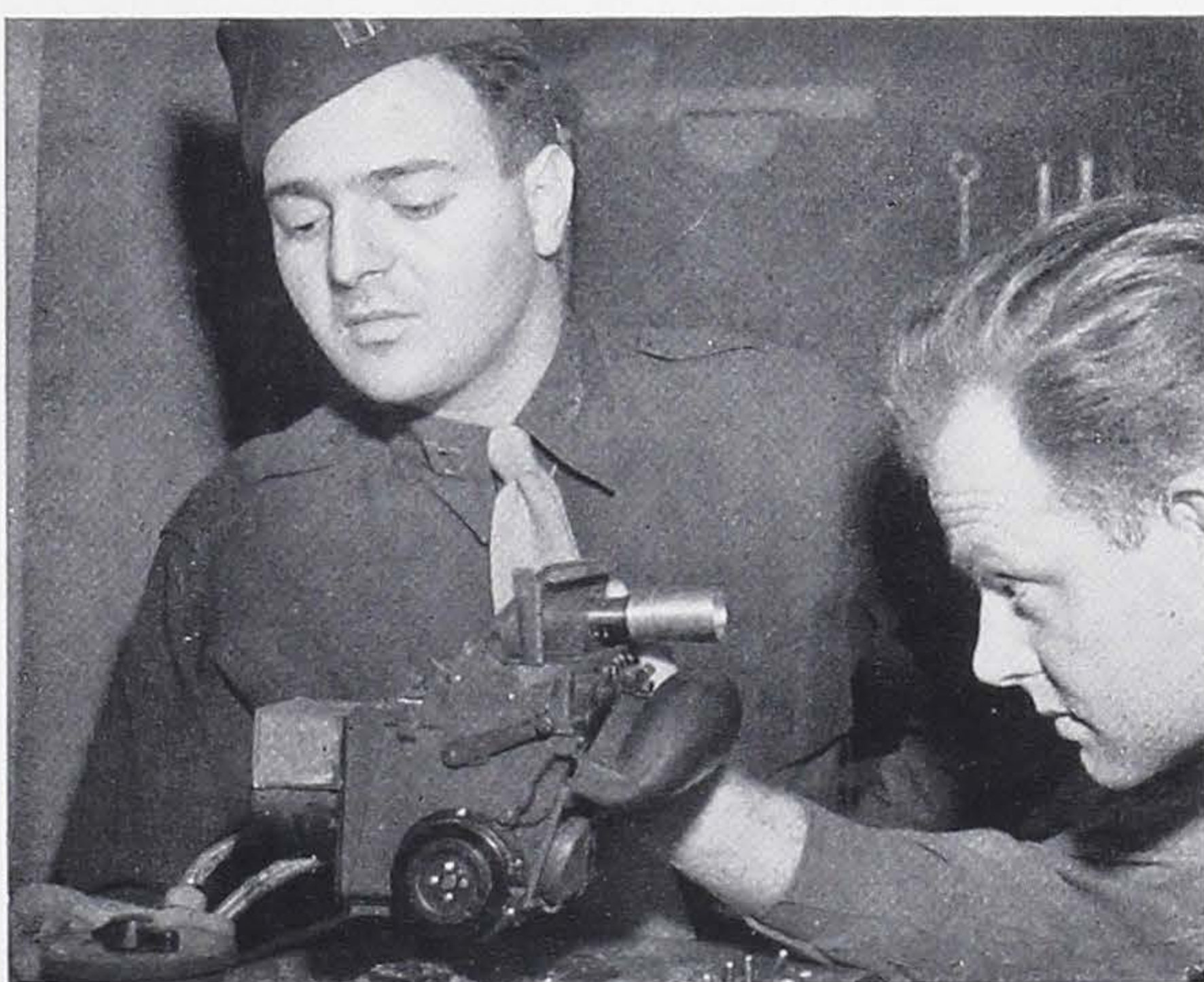
Captain Louis Vacca regulates a gyro gunsight tester as Sgt Merrick Hall checks the instrument. Ordnance and armament section was responsible for keeping an adequate supply of such materials to keep the groups functioning properly.
